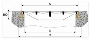
Use of T section frames of 750 mm: **reference E7** T section frames with planarity betweens edges 2 mm and linearity 1 mm Concrete strength  $\geq$  10 MPa
