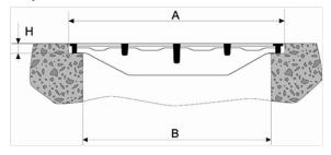
Planarity between edges 2 mm and linearity 1 mm. Concrete strength ≥ 15 MPa
