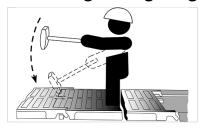
The gratings are easy to install. They are simply snapped into place through a ductile spring lock. The spring bar of the last grating must not be at the extremity of the channel.
